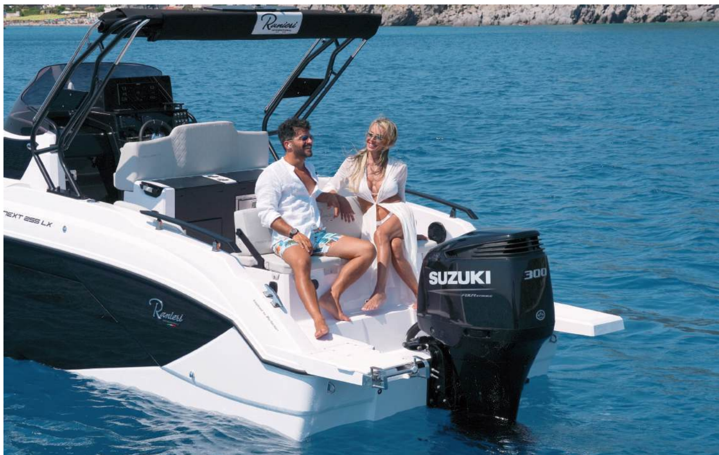
The Suzuki DF300AP is equipped with a 4.028 cc DOHC 6-cylinder engine, delivering 300 horsepower and 4 valves per cylinder.
